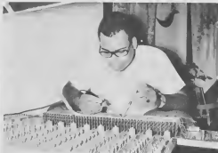
One of the most time-consuming jobs is the soldering of numerous wires. Here Hendrik works on the soundbox with soldering gun and pliers.
